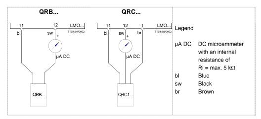
As an alternative to detector current measurement, the diagnostic tool OCI400 / ACS410 can be used. In that case, connection of the DC microammeter is not required.
